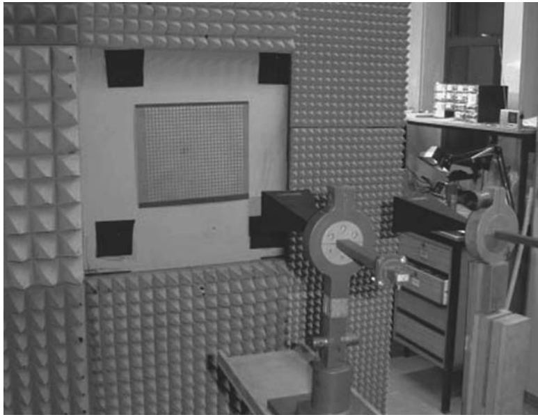
FIGURE 31.9 Experimental setup for testing the AMC performance.
